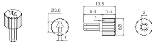
The arrow is in line with the wiper when potentiometer has rotor J (with M rotor, there is a 30° difference).
