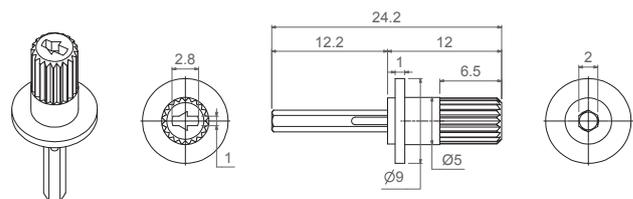
Thumbwheels are available in different colors (color chart in "how to order" section) and with self-extinguishable property according to UL 94 V-0, under request. Thumbwheels can be mounted on the potentiometers at ACP or sold separately. ACP can study special thumbwheel designs.
