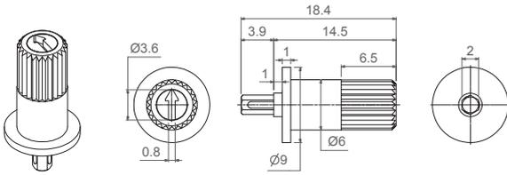
The arrow is in line with the wiper when potentiometer has rotor J (with M rotor, there is a 30° difference).
