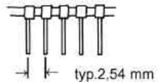
Ø hole in PCB typ. 1,0 mm
