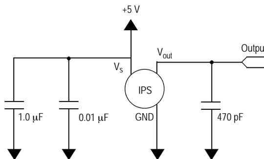
Figure 4. Recommended Power Supply Decoupling and Output Filtering
