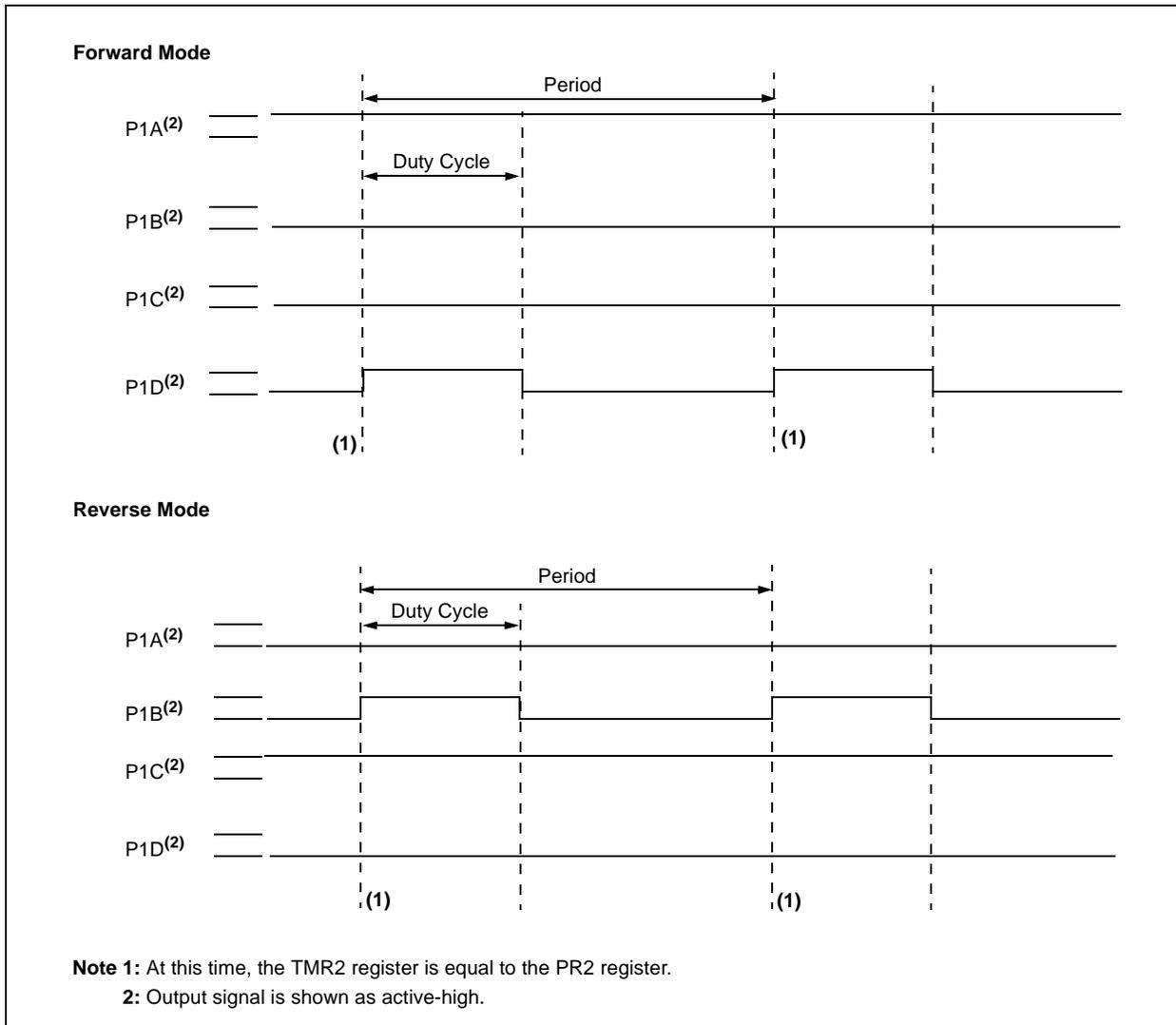
**FIGURE 16-7: EXAMPLE OF FULL-BRIDGE APPLICATION**
