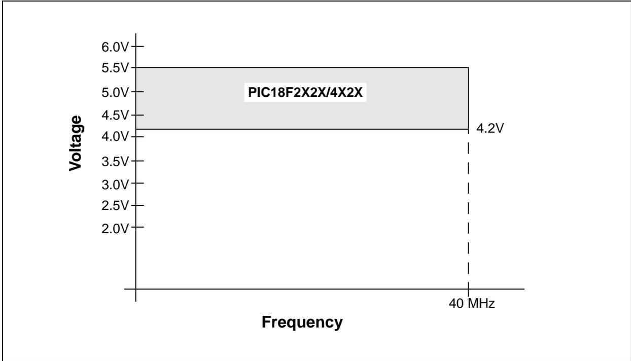
FIGURE 26-2: PIC18F2220/2320/4220/4320 VOLTAGE-FREQUENCY GRAPH (EXTENDED)
