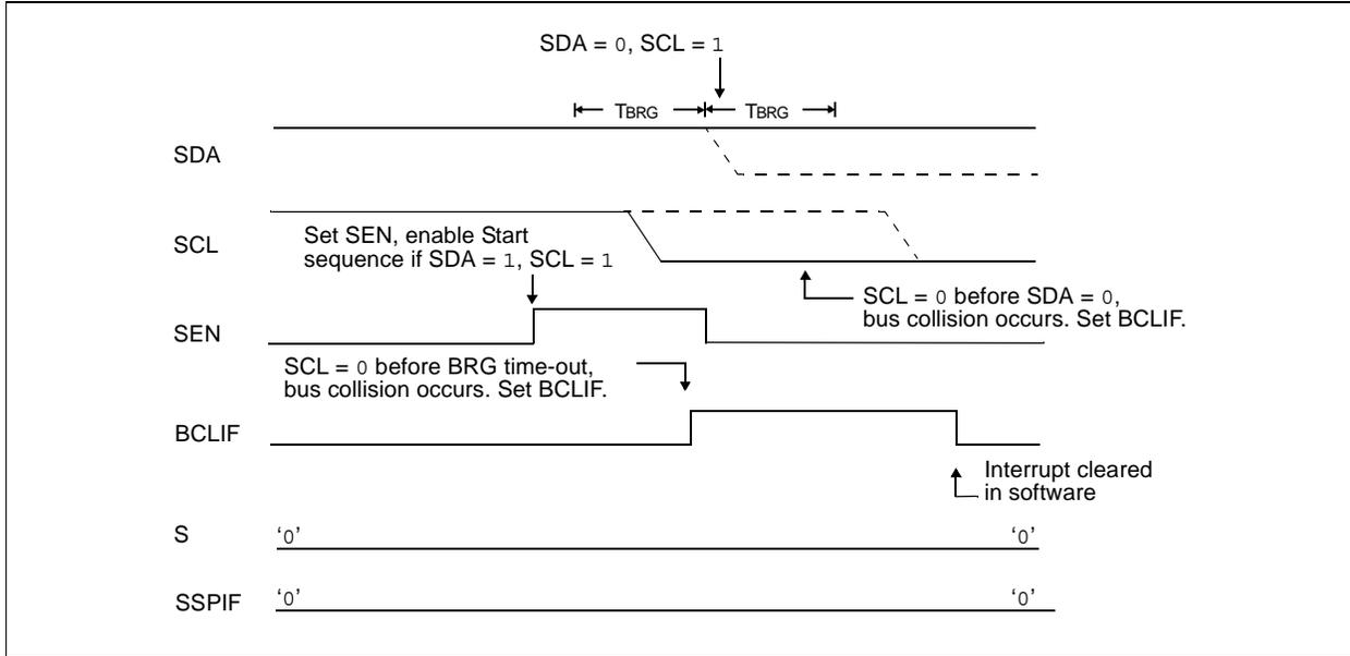
**FIGURE 17-28: BRG RESET DUE TO SDA ARBITRATION DURING START CONDITION**
