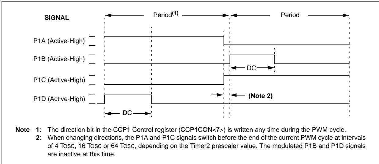
**FIGURE 16-9: PWM DIRECTION CHANGE AT NEAR 100% DUTY CYCLE**
