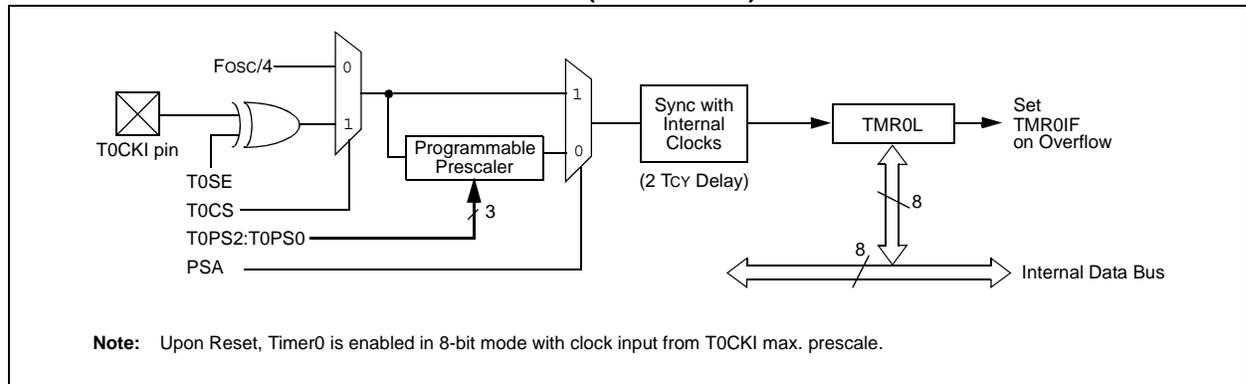
**FIGURE 11-2: TIMER0 BLOCK DIAGRAM (16-BIT MODE)**
