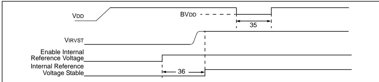
**TABLE 26-10: RESET, WATCHDOG TIMER, OSCILLATOR START-UP TIMER, POWER-UP TIMER AND BROWN-OUT RESET REQUIREMENTS**
