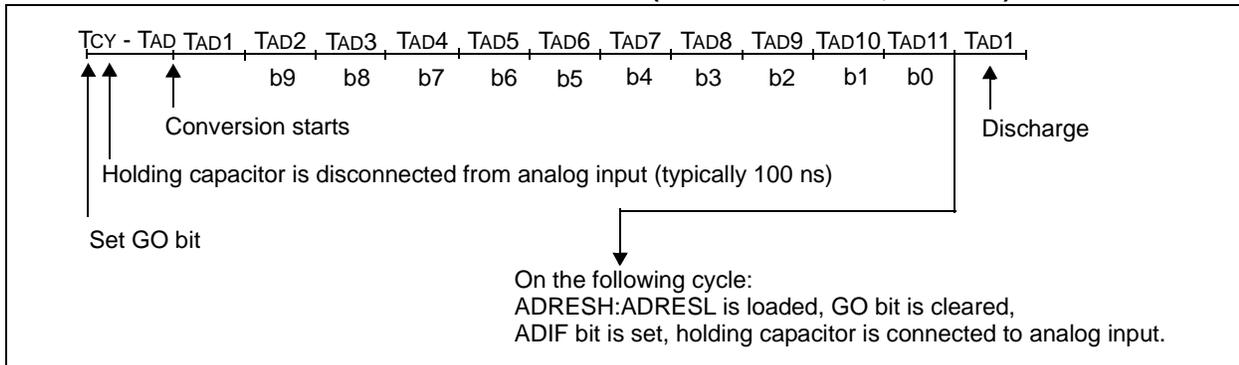
**FIGURE 19-5: A/D CONVERSION TAD CYCLES (ACQT<2:0> = 010, TACQ = 4 TAD)**
