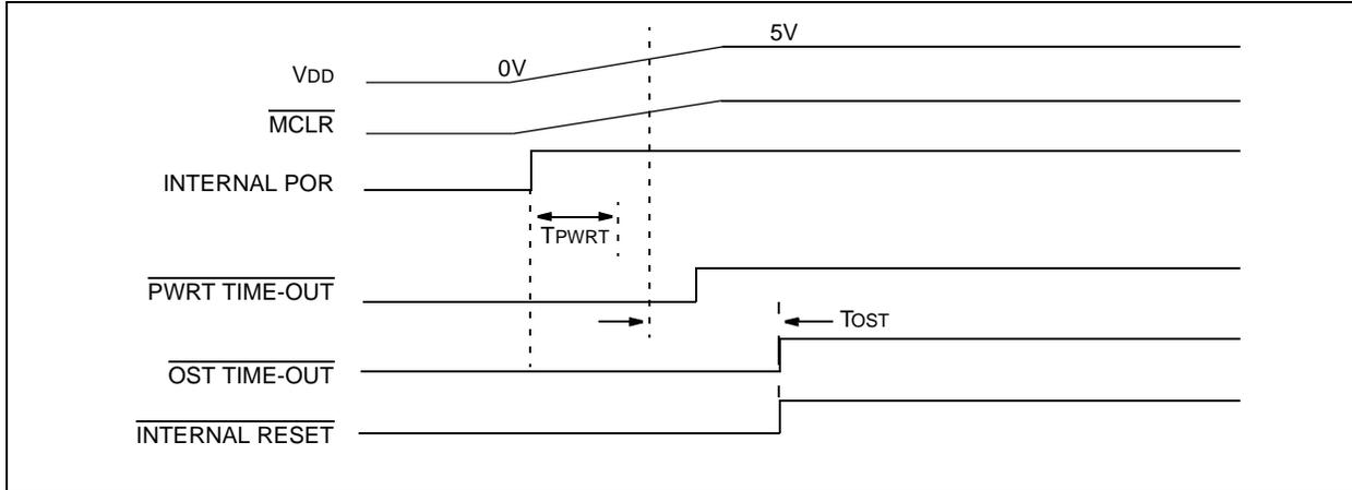
**FIGURE 4-7: TIME-OUT SEQUENCE ON POR W/PLL ENABLED ( $\overline{\text{MCLR}}$  TIED TO  $V_{\text{DD}}$ )**
