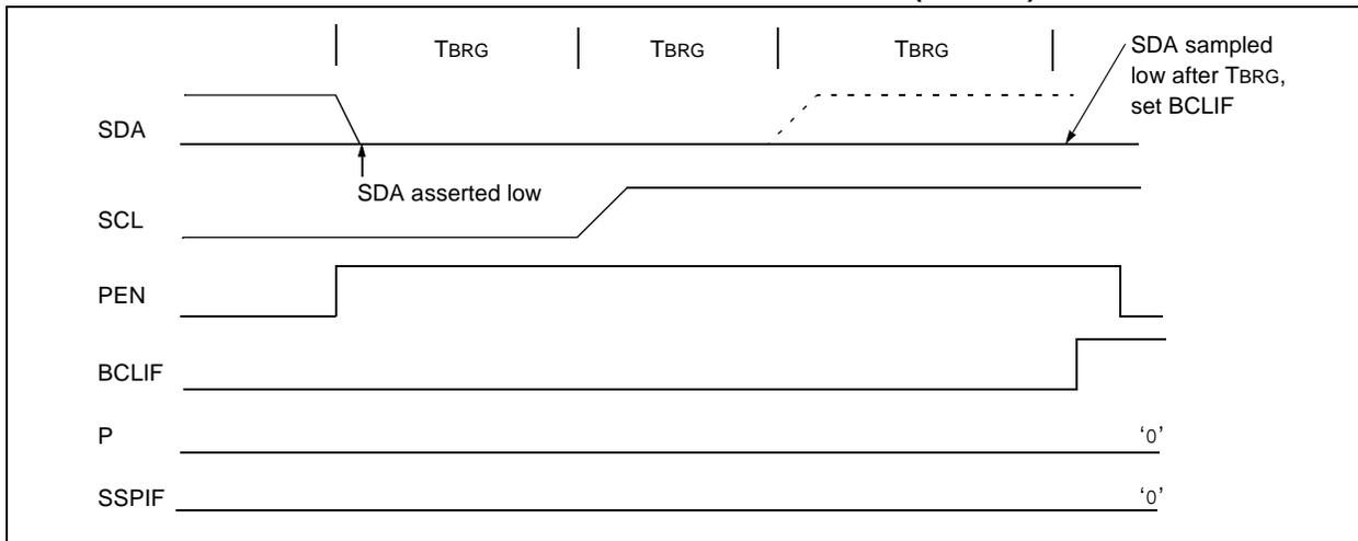
**FIGURE 17-32: BUS COLLISION DURING A STOP CONDITION (CASE 2)**
