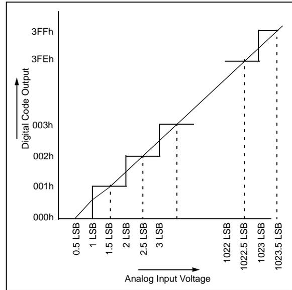
**FIGURE 19-3: ANALOG INPUT MODEL**
