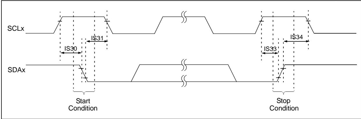
**FIGURE 24-16: I2Cx BUS DATA TIMING CHARACTERISTICS (SLAVE MODE)**
