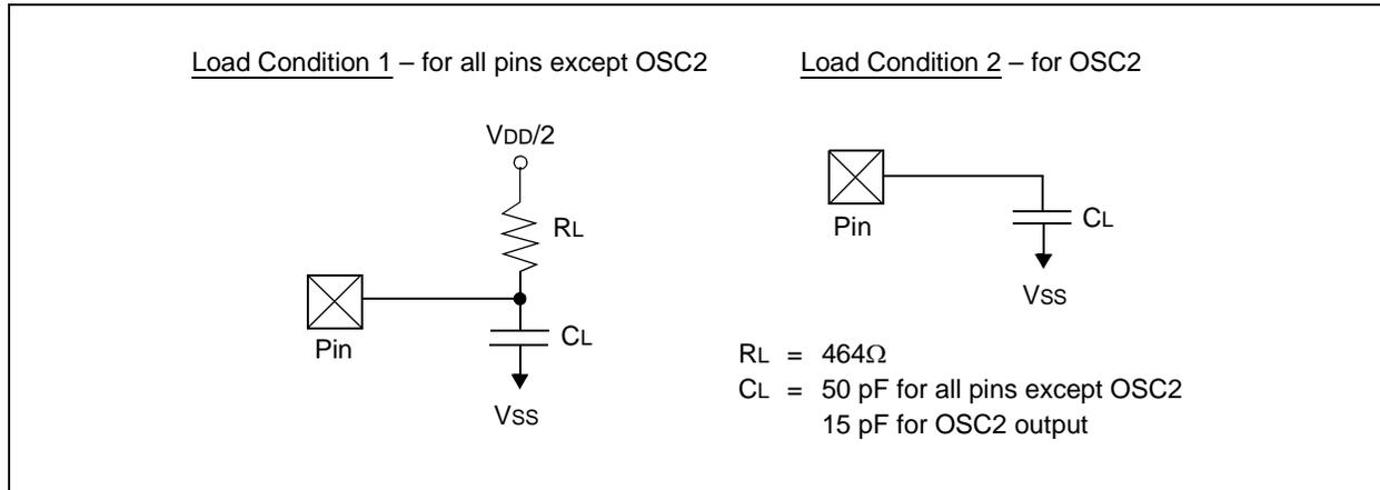
**TABLE 24-15: CAPACITIVE LOADING REQUIREMENTS ON OUTPUT PINS**
