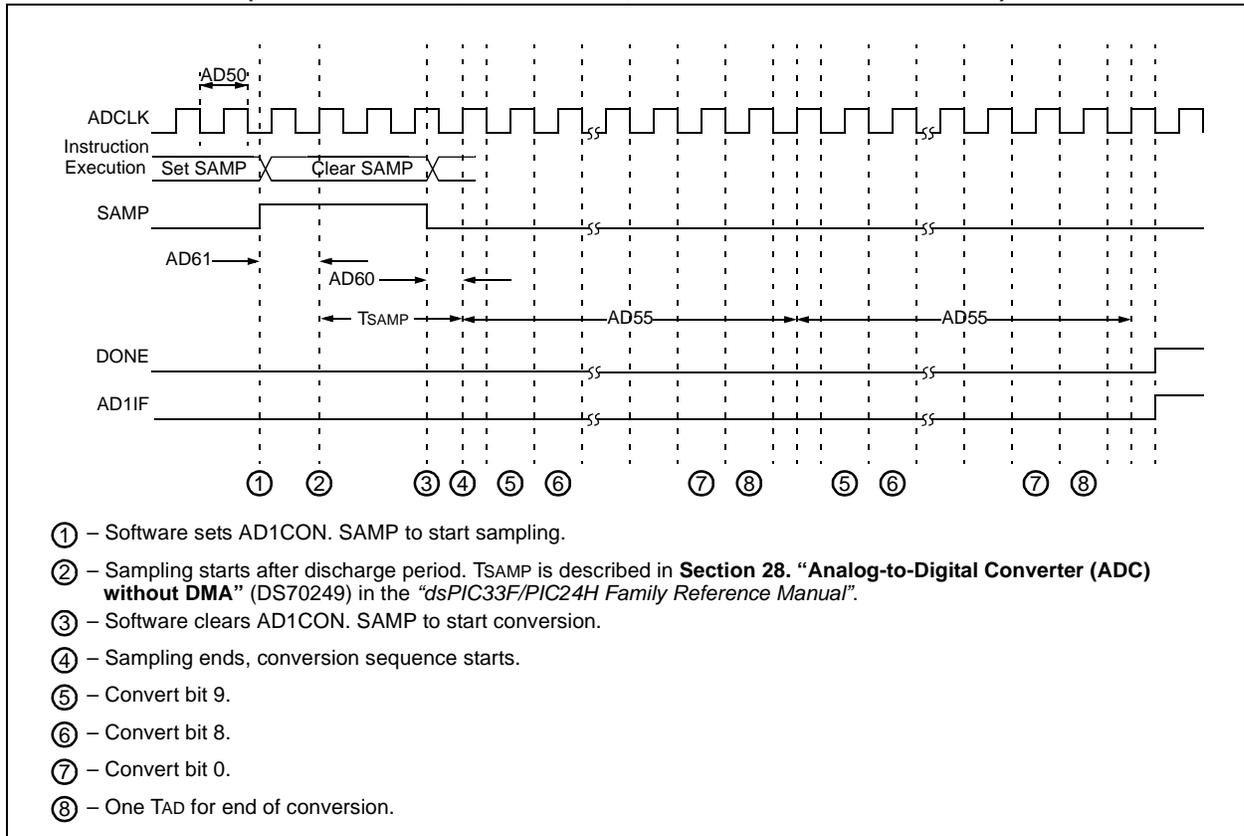
**FIGURE 24-20: ADC CONVERSION (10-BIT MODE) TIMING CHARACTERISTICS (CHPS<1:0> = 01, SIMSAM = 0, ASAM = 1, SSRC<2:0> = 111, SAMC<4:0> = 00001)**
