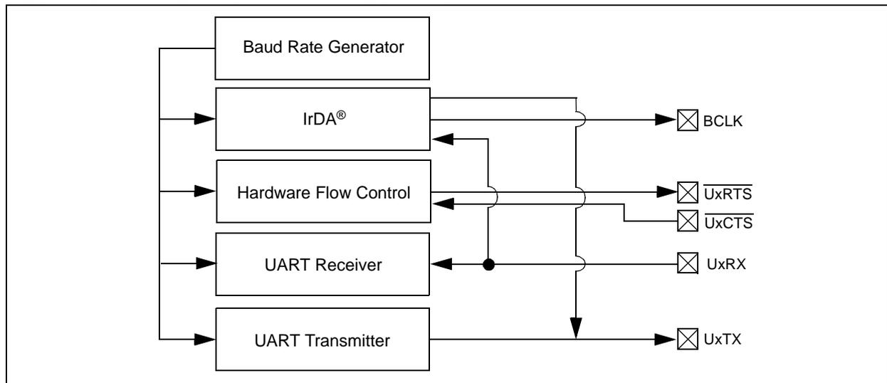
**Note 1:** Both UART1 and UART2 can trigger a DMA data transfer. If U1TX, U1RX, U2TX or U2RX is selected as a DMA IRQ source, a DMA transfer occurs when the U1TXIF, U1RXIF, U2TXIF or U2RXIF bit gets set as a result of a UART1 or UART2 transmission or reception.
