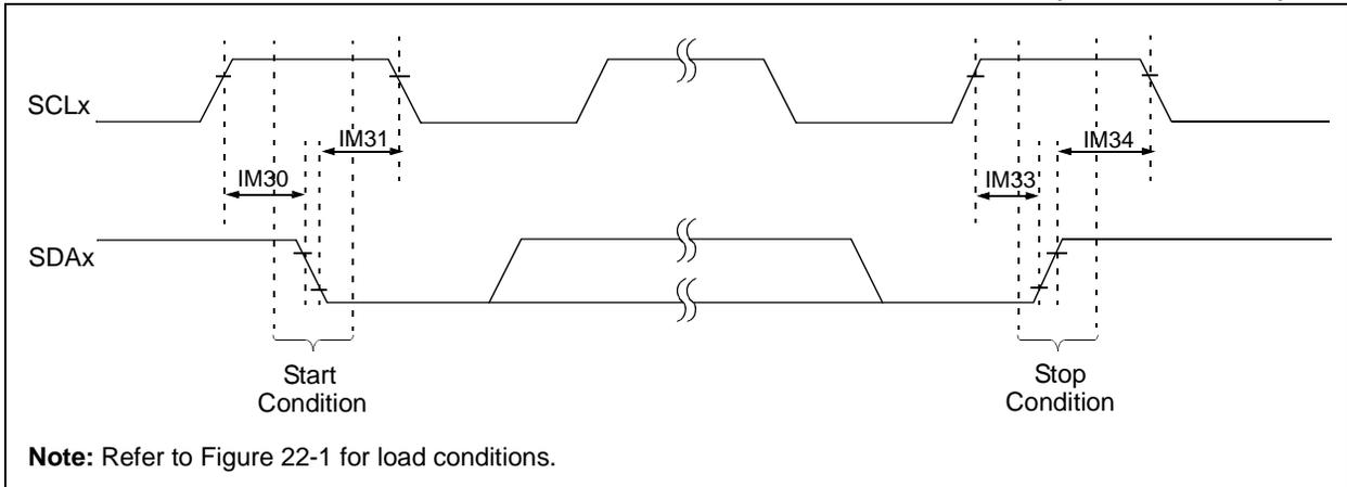
**FIGURE 22-14: I2Cx BUS DATA TIMING CHARACTERISTICS (MASTER MODE)**
