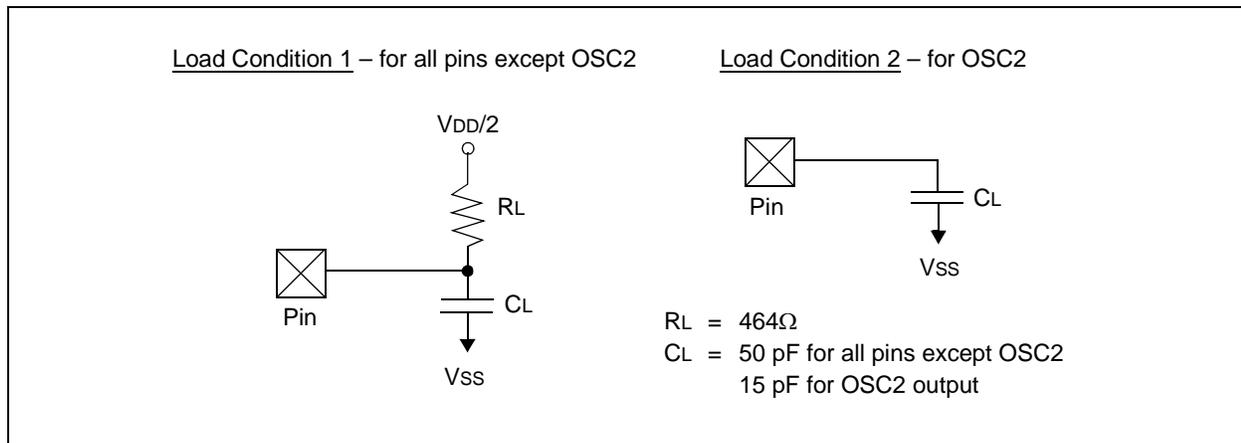
**TABLE 22-15: CAPACITIVE LOADING REQUIREMENTS ON OUTPUT PINS**
