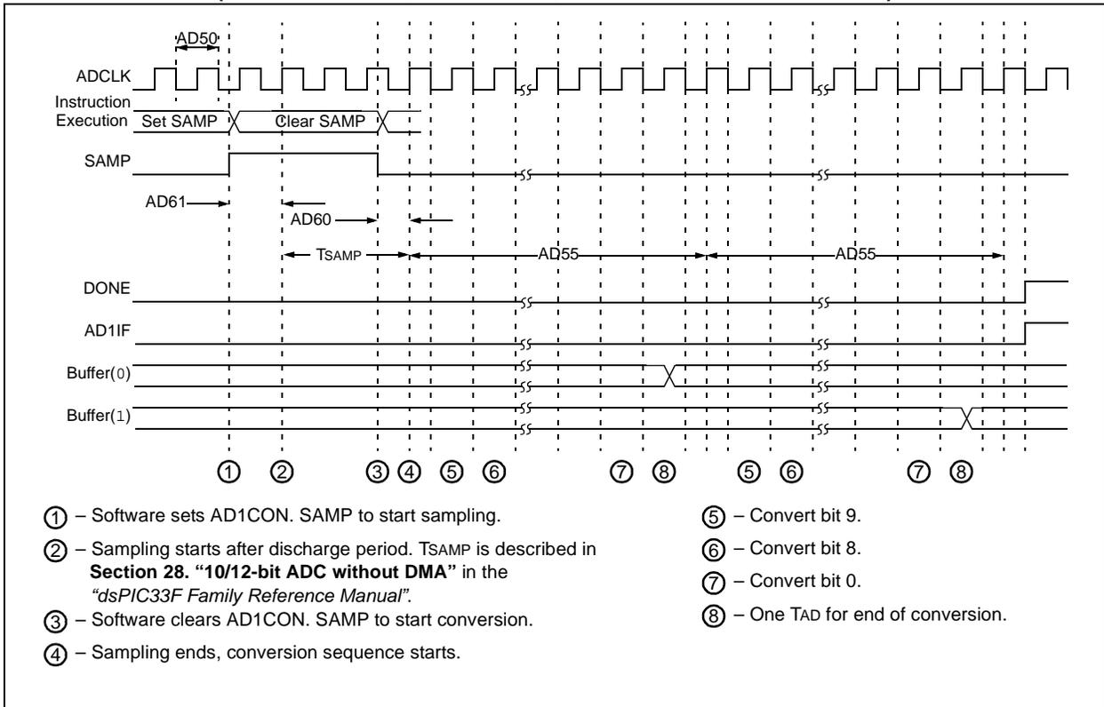
**FIGURE 22-19: ADC CONVERSION (10-BIT MODE) TIMING CHARACTERISTICS (CHPS<1:0> = 01, SIMSAM = 0, ASAM = 1, SSRC<2:0> = 111, SAMC<4:0> = 00001)**
