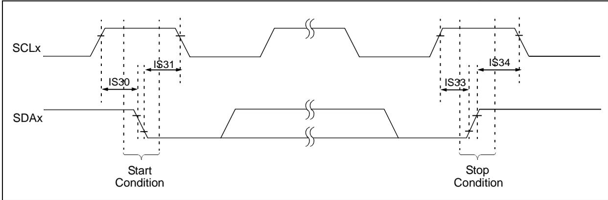
FIGURE 22-16: I2Cx BUS DATA TIMING CHARACTERISTICS (SLAVE MODE)
