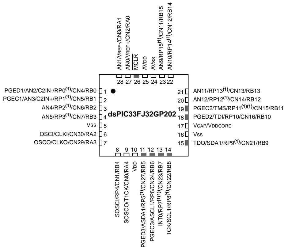
**Note 1:** The RPN pins can be used by any remappable peripheral. See Table 1 for the list of available peripherals.
