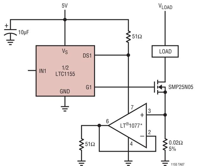
\*DO NOT SUBSTITUTE. MUST BE A PRECISION, SINGLE SUPPLY, MICROPOWER OP AMP ( $I_q < 60\mu A$ )
