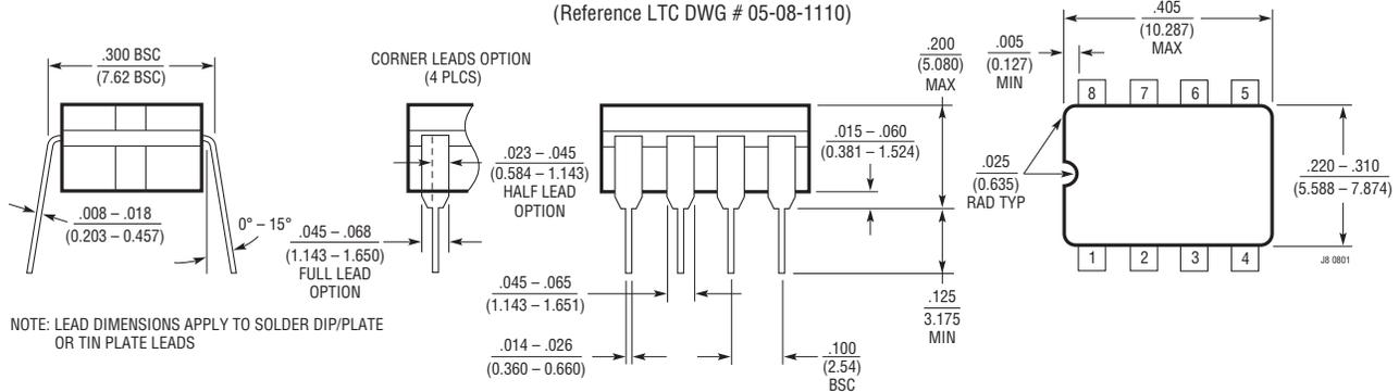
NOTE: LEAD DIMENSIONS APPLY TO SOLDER DIP/PLATE OR TIN PLATE LEADS
