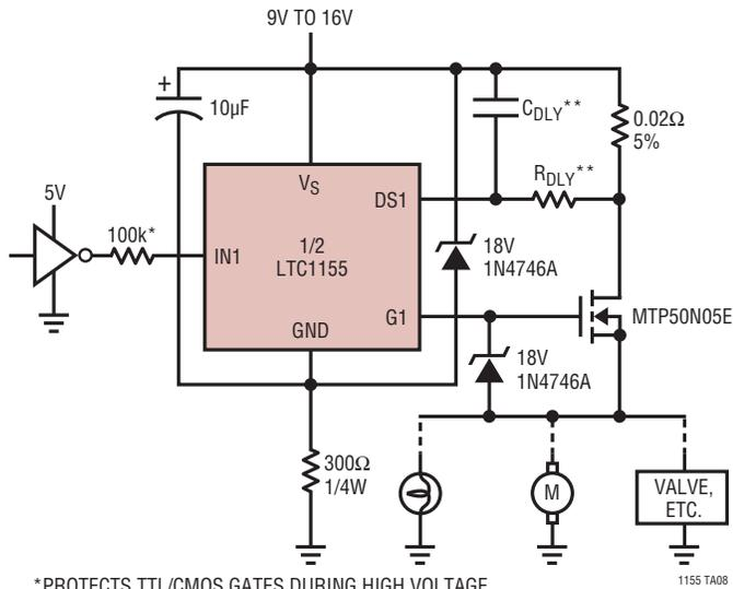
\*PROTECTS TTL/CMOS GATES DURING HIGH VOLTAGE TRANSIENT OR REVERSE BATTERY
