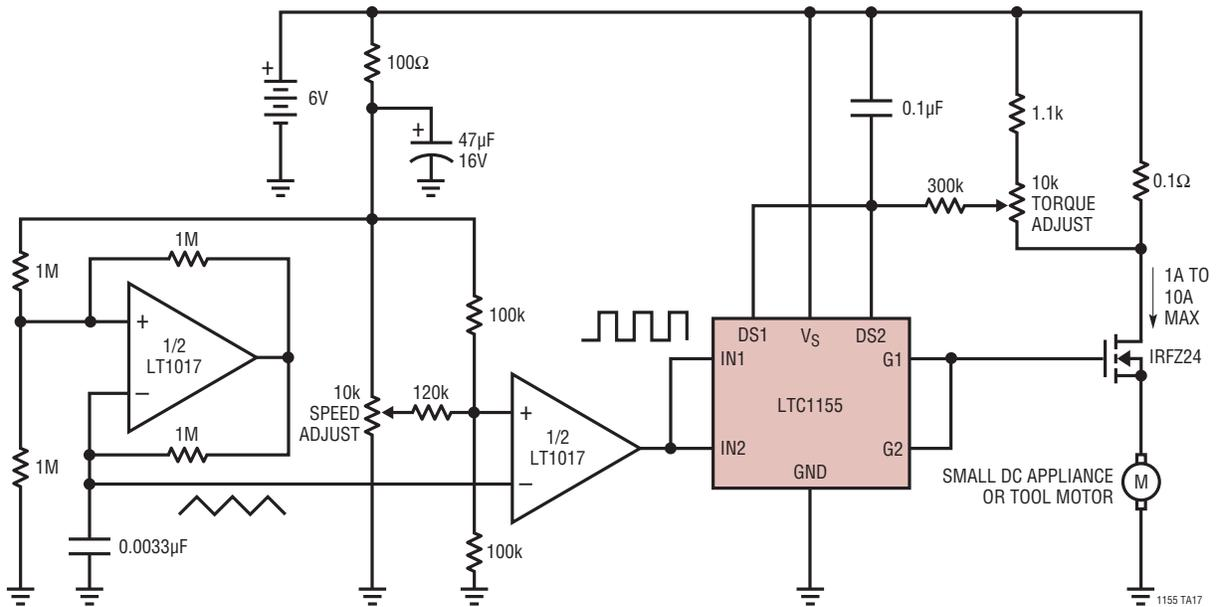
SPEED IS PROPORTIONAL TO PULSE WIDTH. TORQUE IS PROPORTIONAL TO CURRENT
