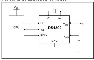
Figure 1. Block Diagram
