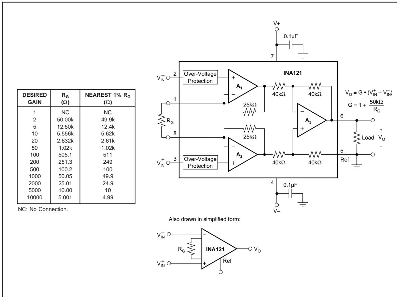
FIGURE 1. Basic Connections.
