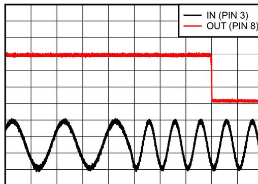
**Figure 13. Frequency Detection**
