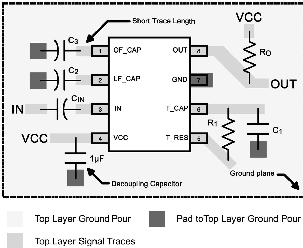
Figure 20. LM567 Layout Example
