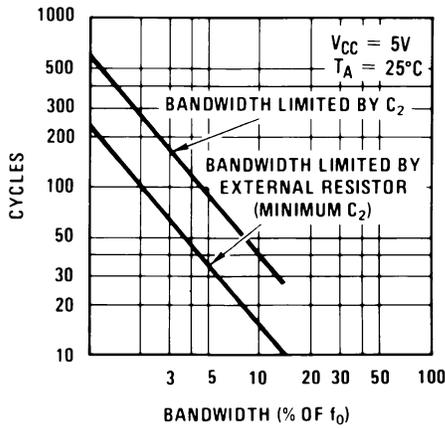
Figure 9. Greatest Number of Cycles Before Output
