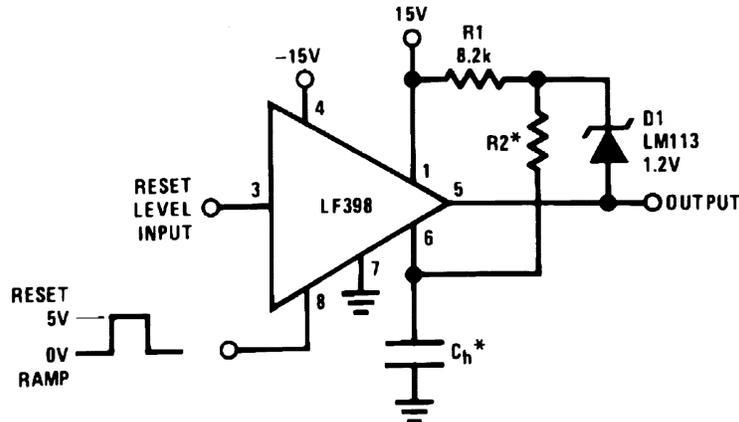
Figure 29. Ramp Generator With Variable Reset Level
