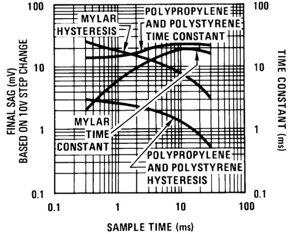
Figure 2. Dielectric Absorption Error in Hold Capacitor
