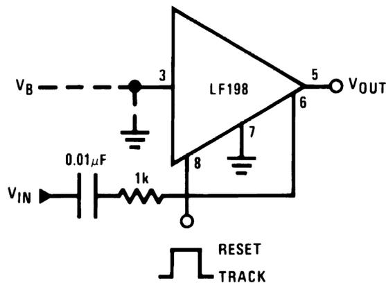
$$V_{OUT} = V_B + \Delta V_{IN} \text{ (HOLD MODE)}$$
