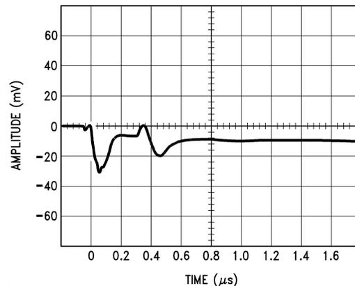
Figure 27. Output Transient at Start of Hold Mode
