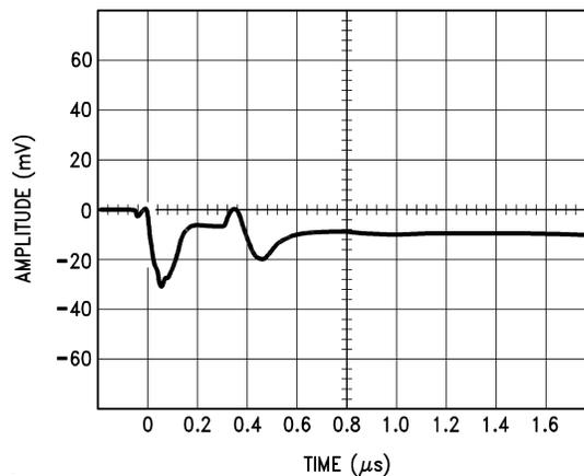
Figure 17. Output Transient at Start of Hold Mode
