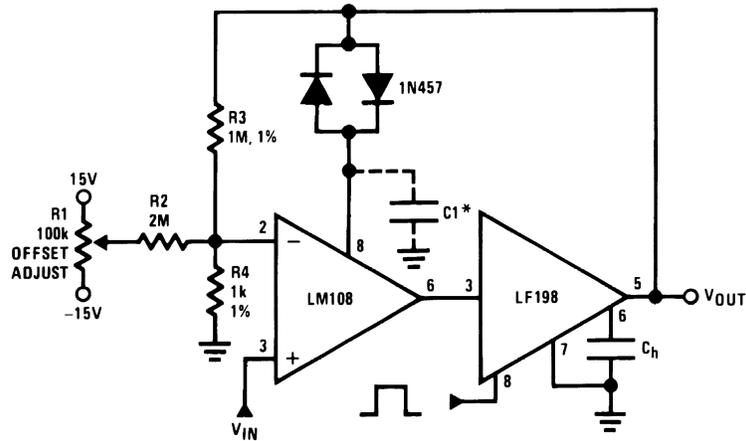
\*For lower gains, the LM108 must be frequency compensated
