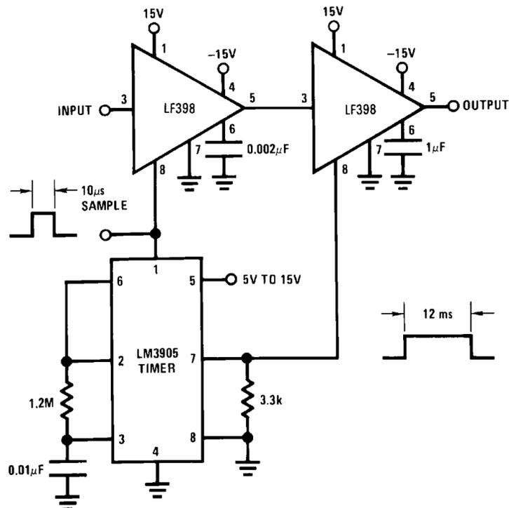
Figure 34. Fast Acquisition, Low Droop Sample and Hold
