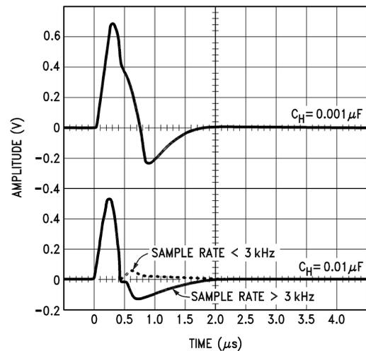
Figure 16. Output Transient at Start of Sample Mode
