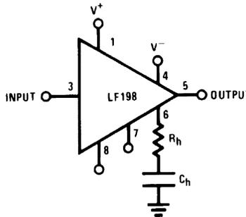
**Figure 31. Output Holds at Average of Sampled Input**
