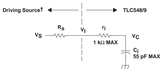
$V_I$  = Input Voltage at ANALOG IN
