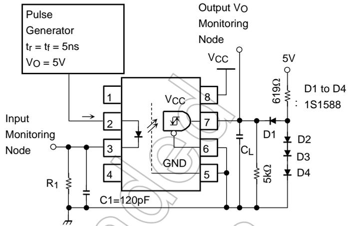
C1 is peaking capacitor. The probe and jig capacitances are included in C1.
