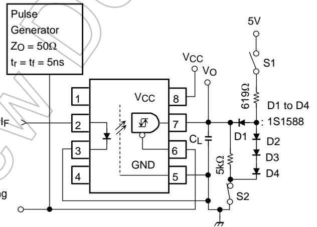
CL is approximately 15pF which includes probe and stray wiring capacitance.
