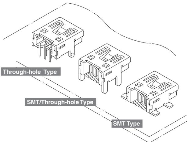
**The USB 2.0 certified receptacle is quite suitable for the interface of the small and miniaturized PC-peripheral products as Digital Cameras and MP3 Players.**
