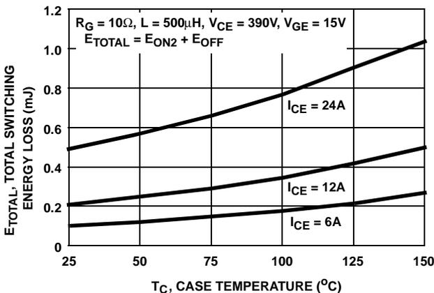
FIGURE 15. TOTAL SWITCHING LOSS vs CASE TEMPERATURE
