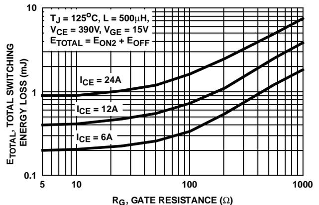
FIGURE 16. TOTAL SWITCHING LOSS vs GATE RESISTANCE
