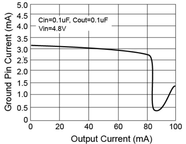
**Figure 4. Ground Pin Current vs. Output Current**
