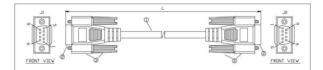
1.CABLE:NO UL.,28AWG(7/0.127),TINNED AND STRANDED COPPER WIRE INSULATOR:PVC,ID:0.85mm ,CABLING:9C+DRAIN WIRE SHIELD:AL/MY COVERAGE
