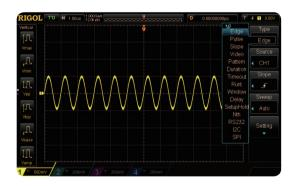
Optional Serial Bus Triggering and Decoding functions(RS232,I2C,SPI)
