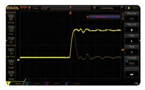
Built in 2 channel 25MHz Signal Source(MSO/DS1000Z-S)
