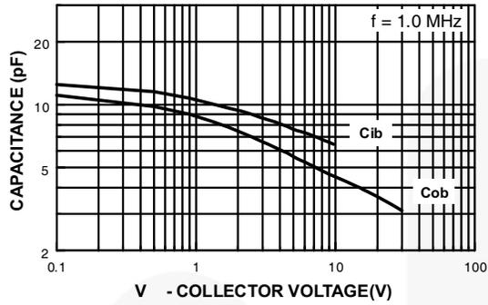
Figure 7. Input and Output Capacitance vs. Reverse Voltage
