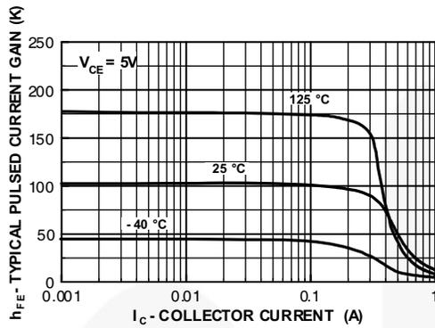
Figure 1. Typical Pulsed Current Gain vs. Collector Current
