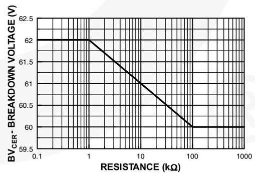
Figure 6. Collector-Emitter Breakdown Voltage with Resistance Between Emitter-Base
