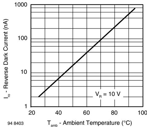
Fig. 1 - Reverse Dark Current vs. Ambient Temperature
