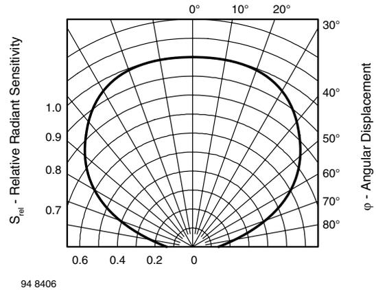
Fig. 7 - Relative Radiant Sensitivity vs. Angular Displacement
