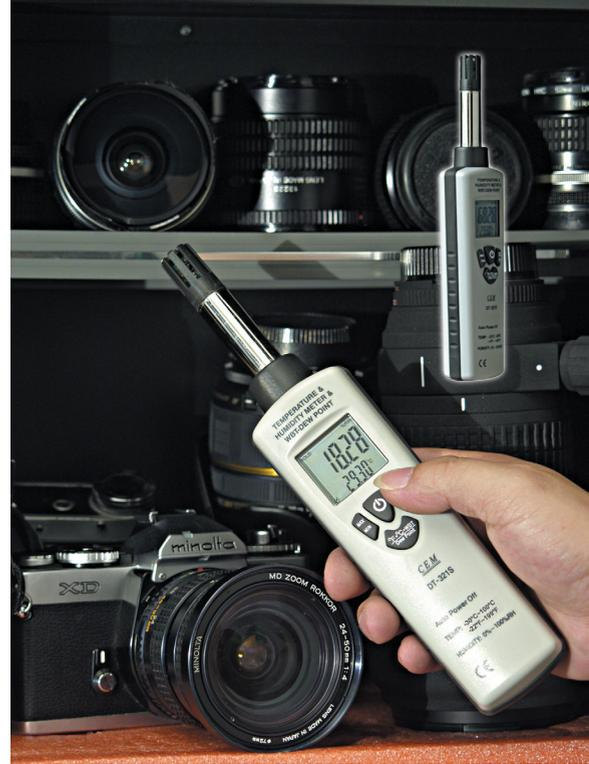
This Humidity & Temperature Meter is for uses a humidity & temperature semiconductor sensor.
