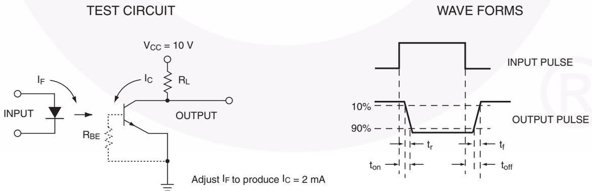
Figure 13. Switching Time Test Circuit and Waveforms
