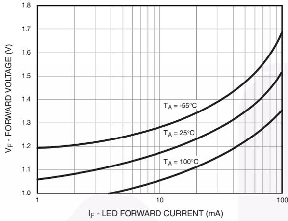
Figure 3. LED Forward Voltage vs. Forward Current
