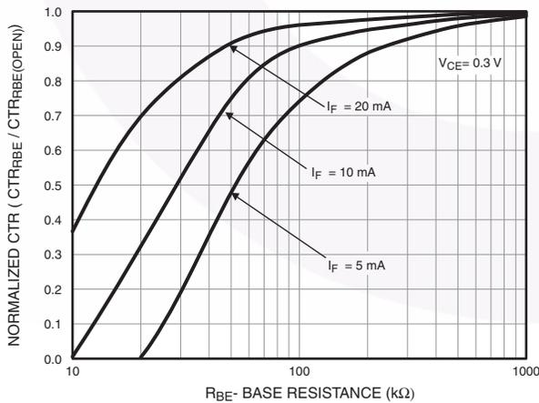
Figure 7. CTR vs. R<sub>BE</sub> (Saturated)
