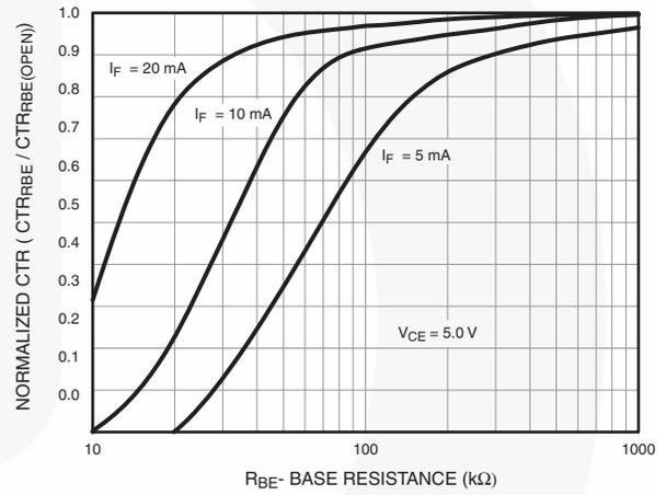
Figure 6. CTR vs. R<sub>BE</sub> (Unsaturated)
