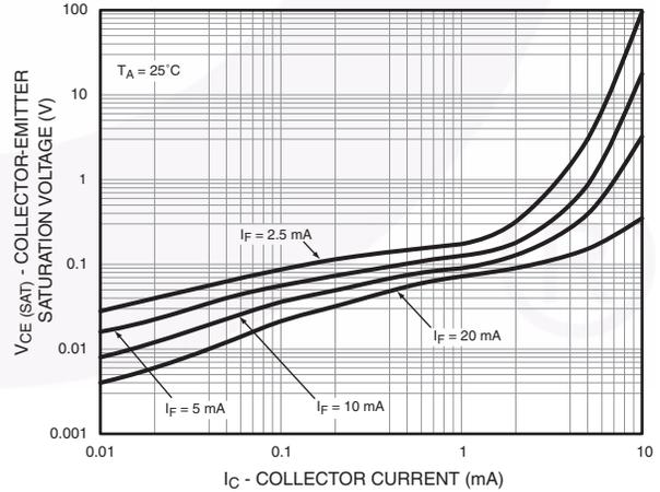
Figure 8. Collector-Emitter Saturation Voltage vs. Collector Current
