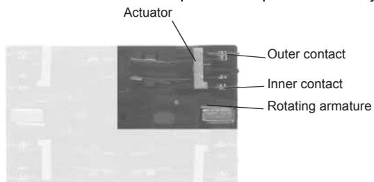
**If an inner contact should weld**, then the movement of the rotating armature is blocked via the actuator.
