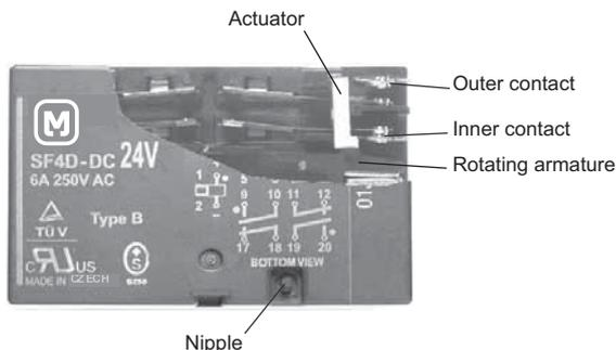
If required a breathing hole can be made in the cover by removing the nipple. However be aware that the degree of protection will reduce from IP67 to IP30!
