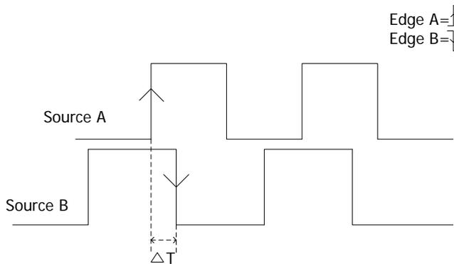
Figure 5-10 Delay Trigger
