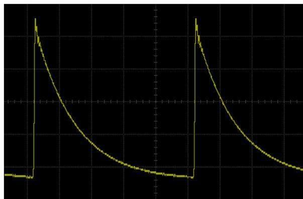
Figure 13-5 Built-in Waveform-ExpFall
