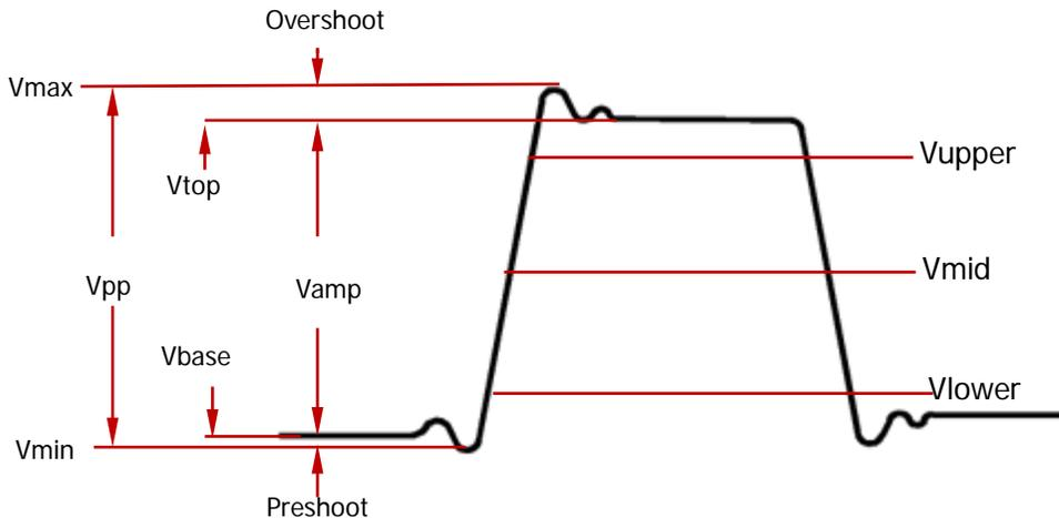
Figure 6-5 Voltage Parameters
