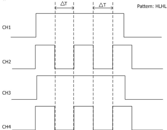
Figure 5-7 Duration Trigger
