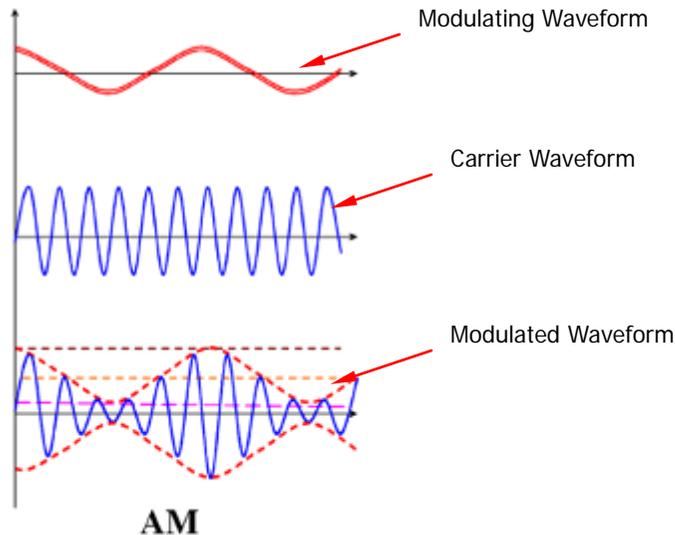
Figure 13-10 Amplitude Modulation
