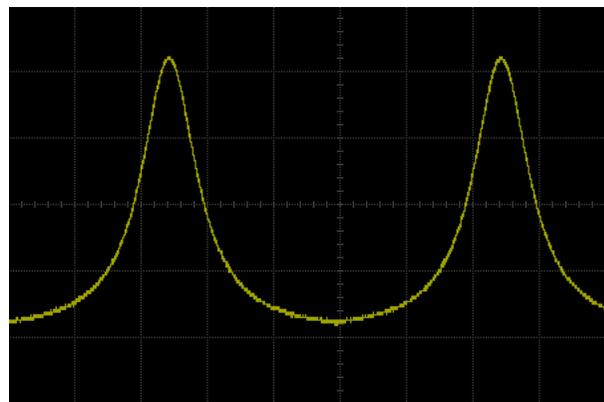
Figure 13-8 Built-in Waveform-Lorentz
