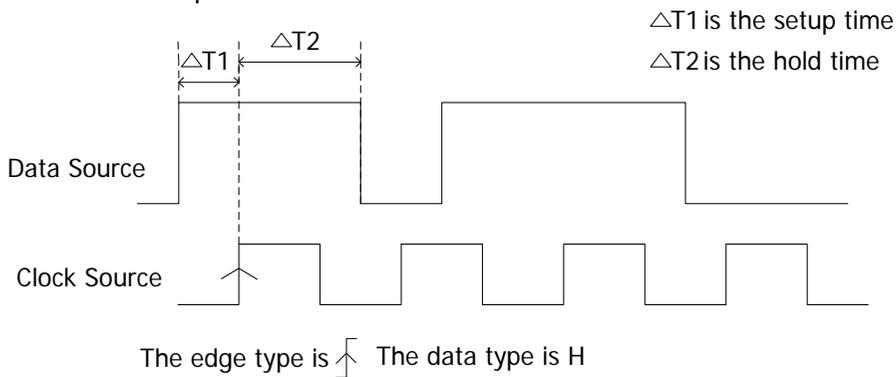
Figure 5-11 Setup/Hold Trigger
