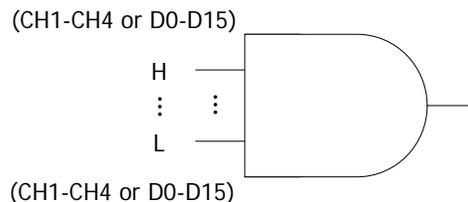
Figure 5-6 Pattern Trigger
