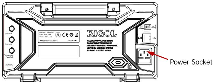
Figure 1-4 To Connect to Power Supply
