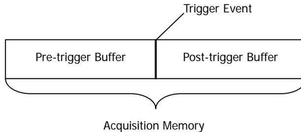
Figure 5-1 Schematic Diagram of the Acquisition Memory
