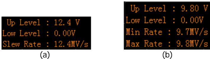
Figure 5-5 Trigger Level Information Display
