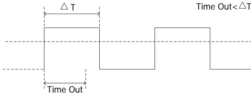
Figure 5-8 TimeOut Trigger
