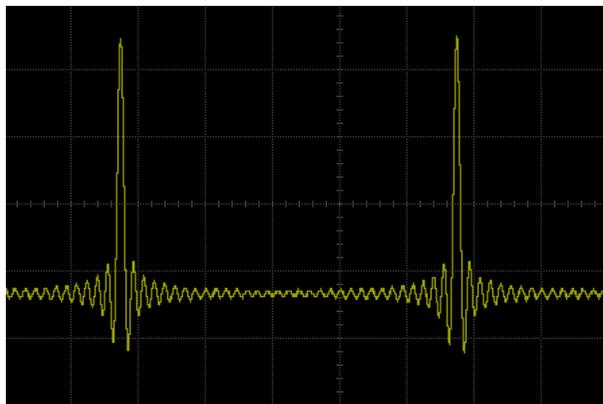
Figure 13-3 Built-in Waveform-Sinc
