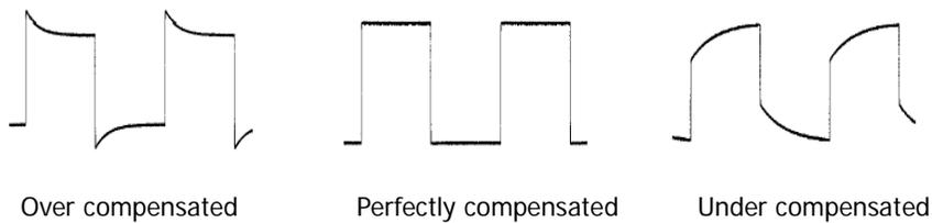
Figure 1-9 Probe Compensation
