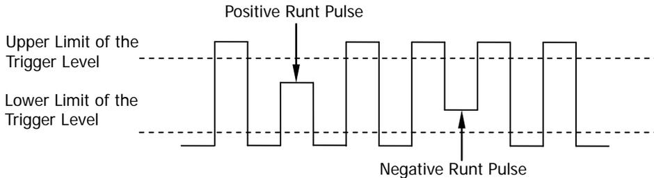
Figure 5-9 Runt Trigger
