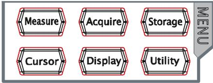
**Measure**: press this key to open the measurement setting menu. You can set the measurement source, turn on or off the frequency counter, all measure, statistic function and etc. Press **MENU** at the left of the screen to open the measurement menus of 33 waveform parameters. Then, press down the corresponding menu softkey to quickly realize one-key measurement and the measurement result will be displayed at the bottom of the screen.
