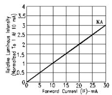
Fig4. RELATIVE LUMINOUS INTENSITY VS. FORWARD CURRENT
